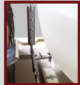
Injection pump inside the cargo box. Air vents prevent heat build-up
