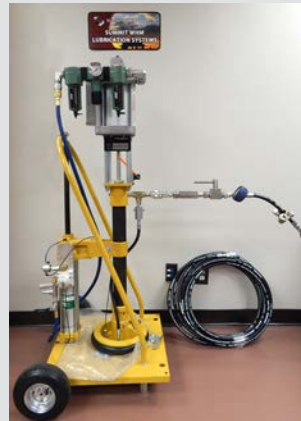
Summit Cart Unit with Single High Pressure (15,000 PSI) High Volume (140:1) grease pump
