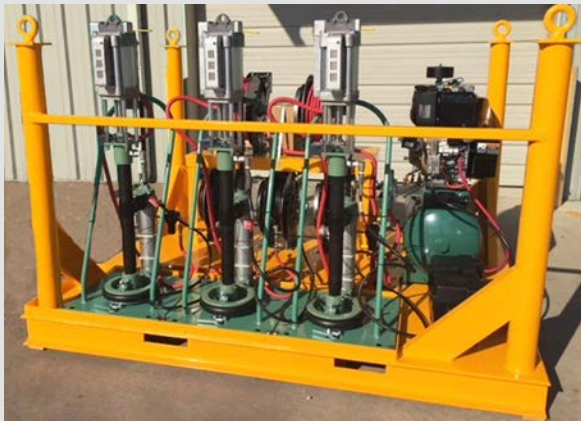
Summit Skid Unit with Multiple High Pressure (15,000 PSI) High Volume (140:1) grease pumps and compressor
